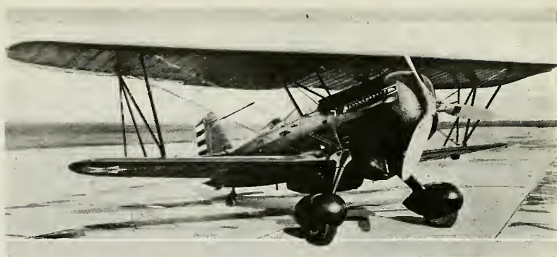
The P6E Curtiss Hawk, Conqueror-powered, with cantilever landing gear
